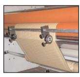
Rotary Trimmers - Available in manual as well as pneumatic versions. These devices are used to remove extra laminate from the side of web or to split web in the web direction. Uses a rotary blade against a hardened anvil roller to create crush cutting action. The blade holder can be positioned laterally with the use
