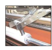
Unwind Slitting – is used to convert a wide roll of film on the unwind shaft to a smaller width web while laminating. The unused material remains on the roll core while the laminating material is introduced into the laminating process. The blade holder is a
