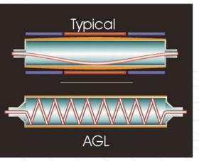
laminator between jobs saving valuable lamination film. Second, AGL uses a silicone coated steel roller construction without a crown. While our competitors use aluminum rollers and crown the silicone coating to compensate for their roller deflection (bending), we know this cost cutting technique will only cause you to have problems like in-feed waves (i.e.where the print buckles going into the laminator causing wrinkles and silvering). AGL rollers are guaranteed to have
