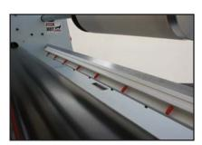
Static Elimination – When static build up from rolls of laminating film creates a hazard for operators; AGL has the solution. The AGL 6400 can be designed to add an optional pulsed DC static elimination bar designed to provide highly
