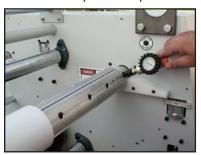
The outside diameter of an air shaft is slightly less than the inside diameter of the core of laminating film that you want to load into the laminator. Once the core of material is in its proper location on the air shaft an inflation tool injects air into a
